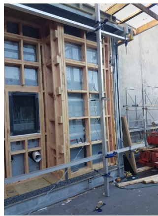
Figure 14: Photo showing location where displacement transducers were placed on full-height timber stud
