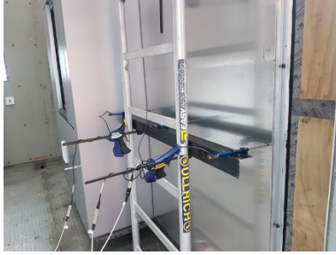
Figure 15: Set of three horizontal transducers setup at the vertical mid-point between stiffeners on a cladding panel.
